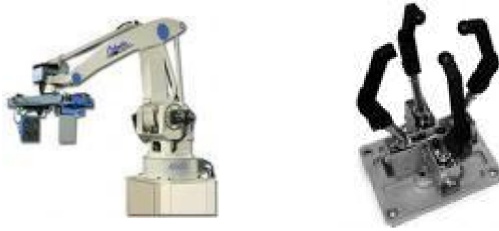
Figure 4.18 Mechanical Gripper
