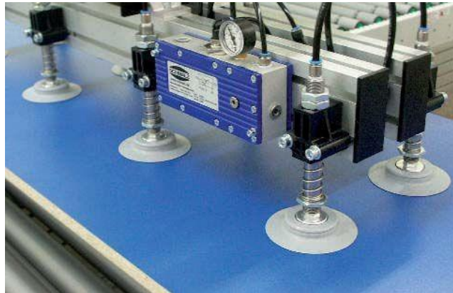
Figure 4.20 Vacuum gripper
