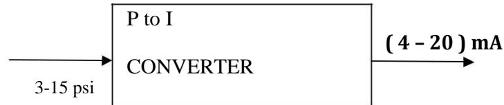
Fig 4.3 P to I converter
