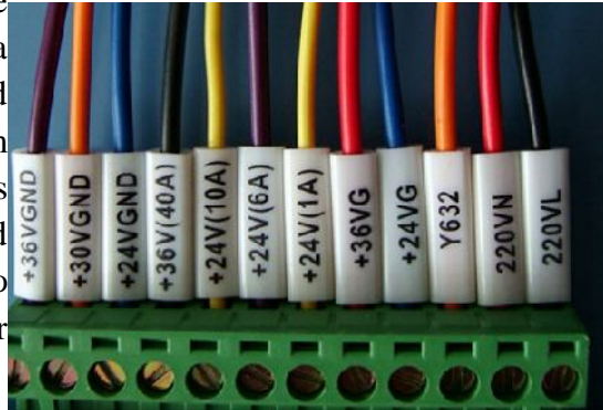
Figure 3.15 Terminal block with Ferules
