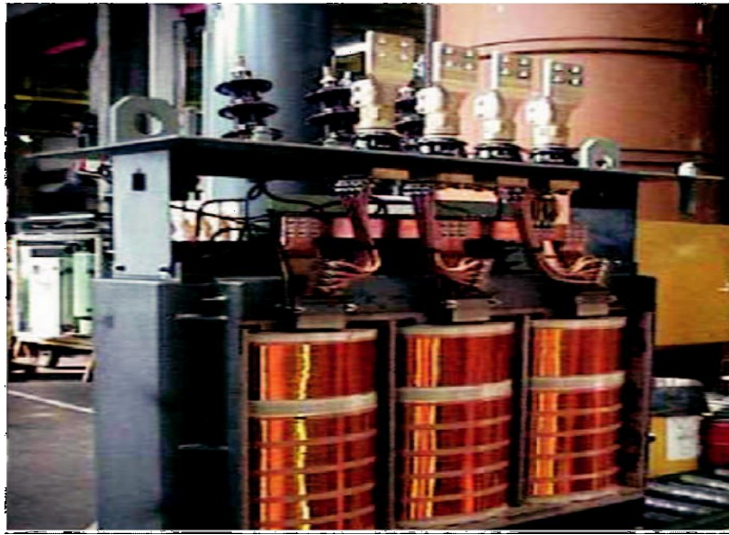
Figure 5.15 1600 kVA Amorphous Core Transformer
