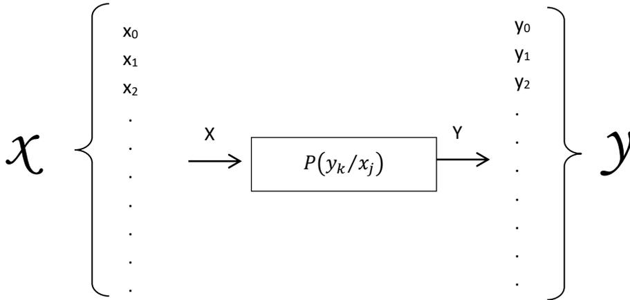
Figure 3.2 Discrete Memoryless channel
