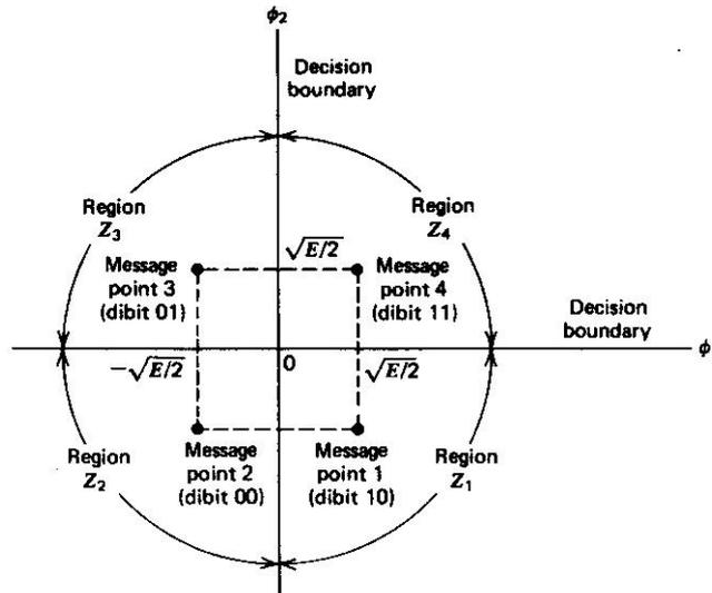
Figure 4.12 Signal space diagram for coherent QPSK system
