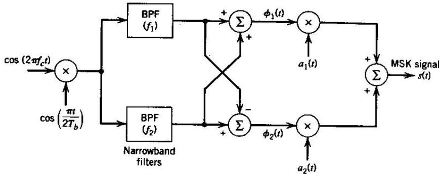
Figure 4.15 Block diagram of MSK transmitter communication system
