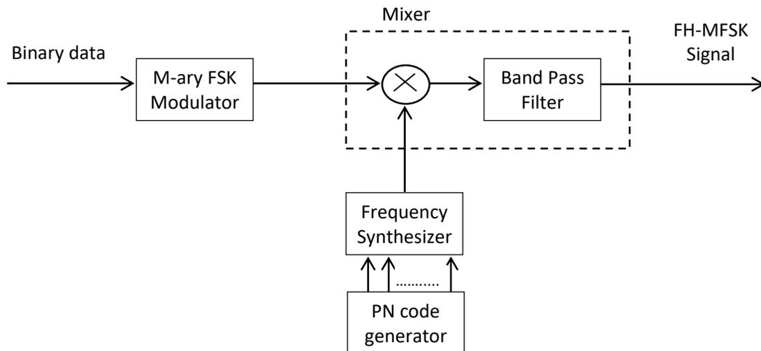
Figure 5.12 FH-MFSK Transmitter
