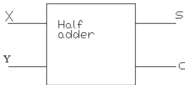
Figure 1.28 Block diagram of half adder
