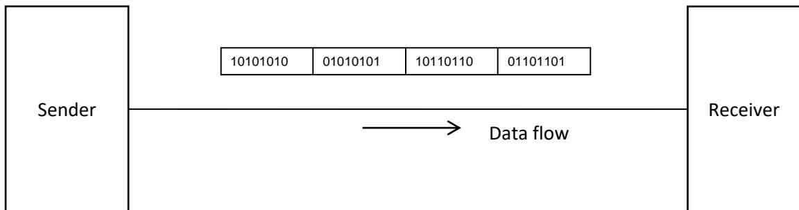
Figure 1.12 Synchronous Transmission
