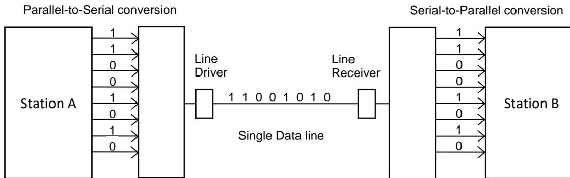
Figure 1.9 Serial Transmission
