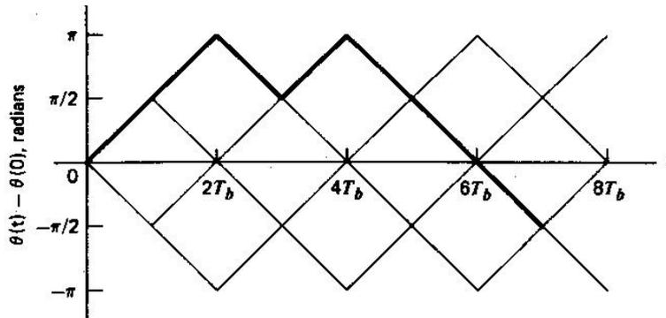
Figure 4.14 phase trellis (for the sequence 1101000)
