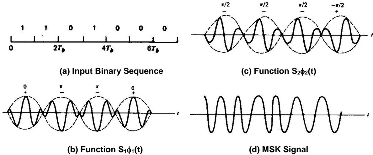
Figure 4.16 sequence and waveforms for MSK signal
