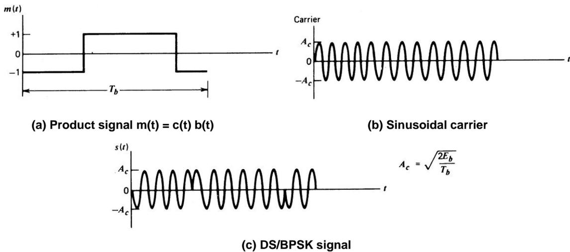
Figure 5.9 Waveforms for Second Stage of Modulation
