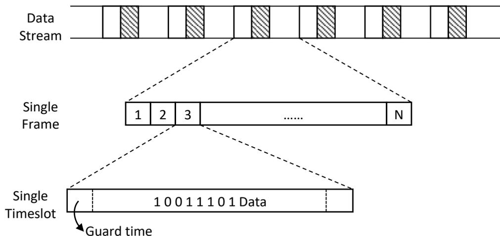
Figure 4.33 TDM Frame structure
