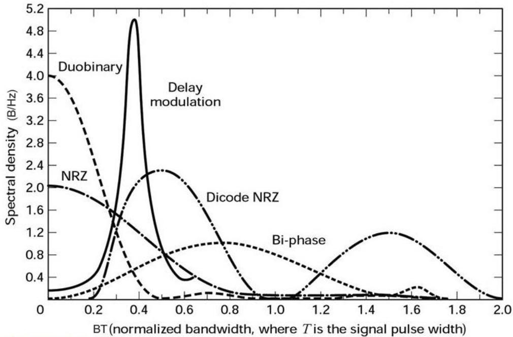
Figure 2.20 Spectral densities of various PCM waveforms
