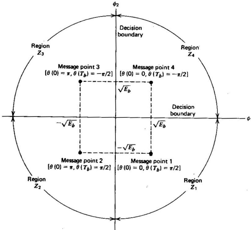
Figure 4.18 signal space diagram for MSK system
