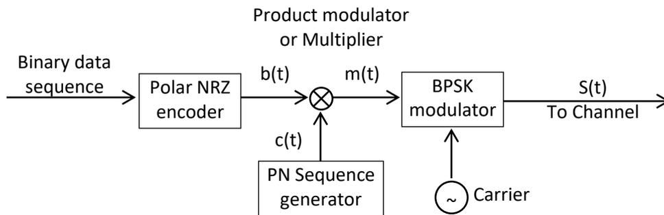
**Figure 5.7 DS-BPSK Transmitter**
