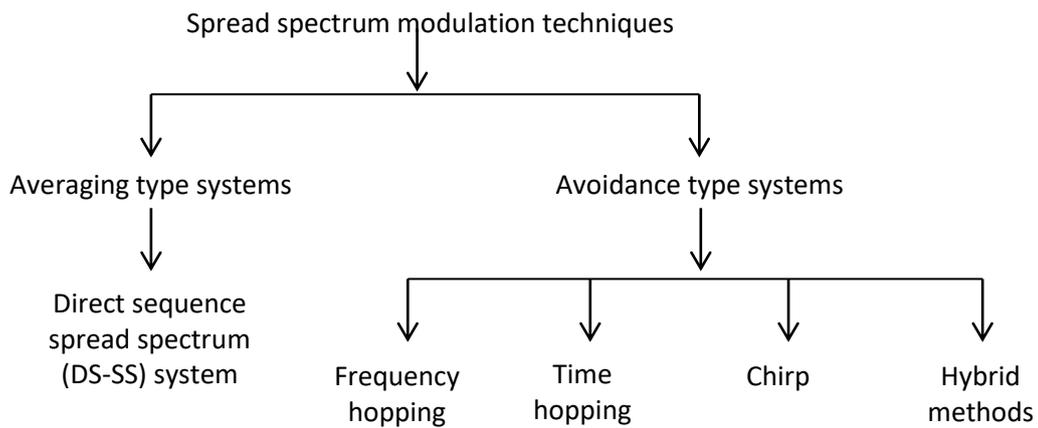
**Figure 5.6 Classification of SS Modulation techniques**
