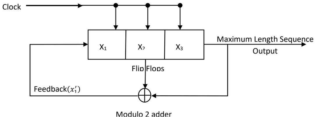
**Figure 5.2 PN sequence or Maximum Length Sequence Generator**
