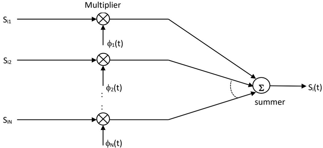
Figure 4.1 Scheme for generating the signal  $S_i(t)$
