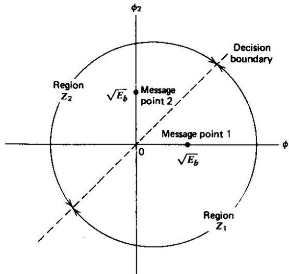
Figure 4.27 signal space diagram for BFSK
