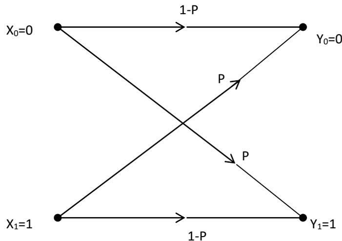
Figure 3.3 Binary Symmetric Channel
