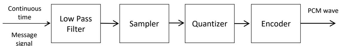
Figure 2.13 PCM transmitter
