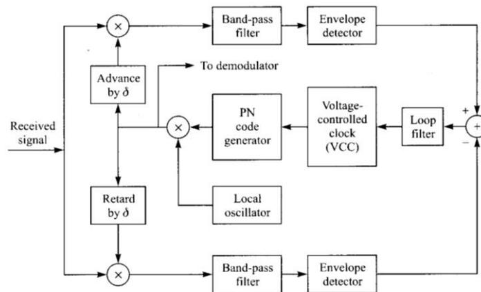
Figure 5.21 Delay-Locked Loop (DLL) for PN code tracking
