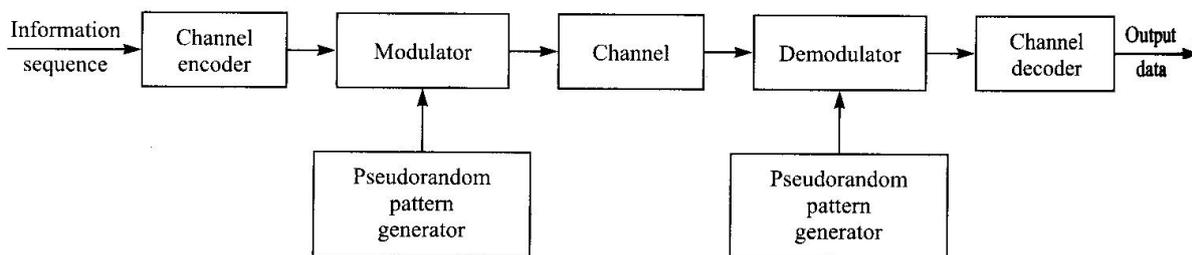
**Figure 5.1 Model of spread spectrum digital communication system**
