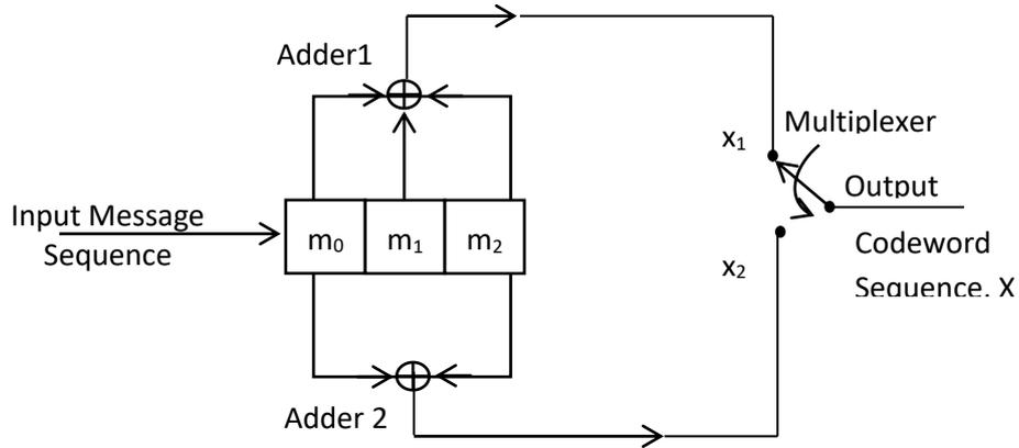
Figure 3.10(b) Convolutional Encoder redrawn alternatively
