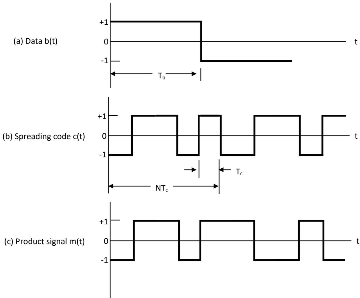
Figure 5.8 Waveforms for First stage of modulation
