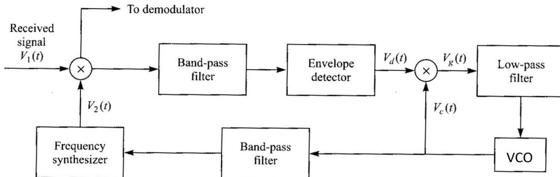
Figure 5.22 Tracking loop for FH signals
