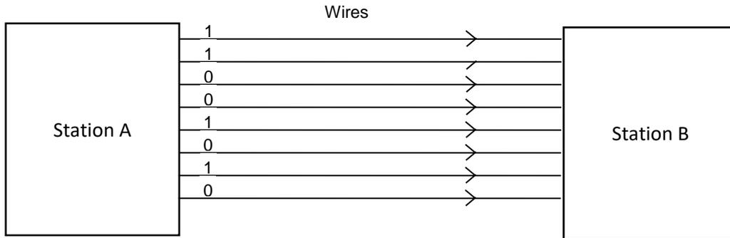
**Figure 1.8 Parallel transmission**
