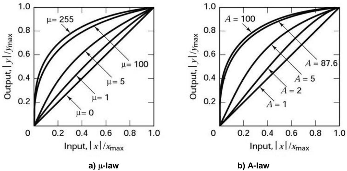
Figure 2.18 Compression Characteristics
