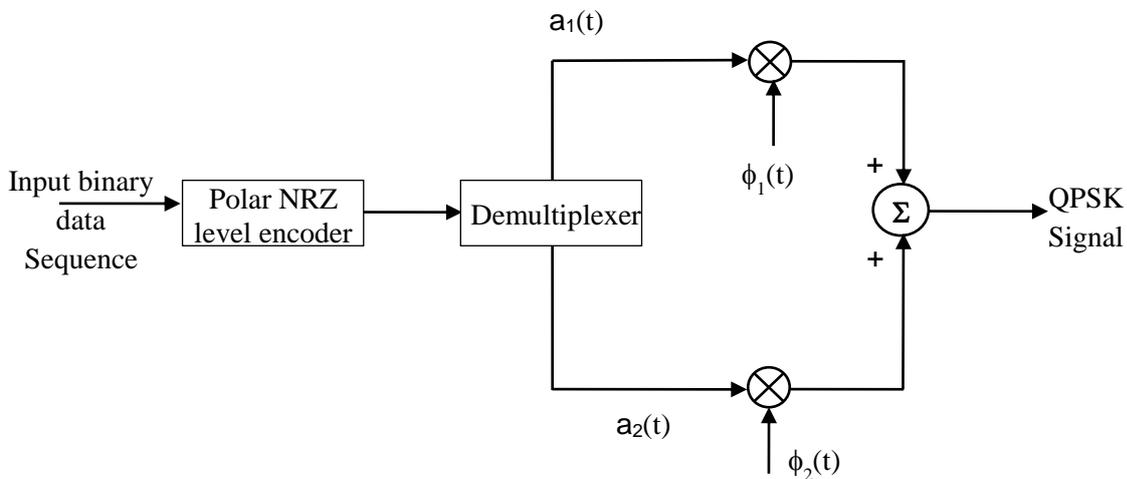
**Figure 4.9 QPSK Transmitter**
