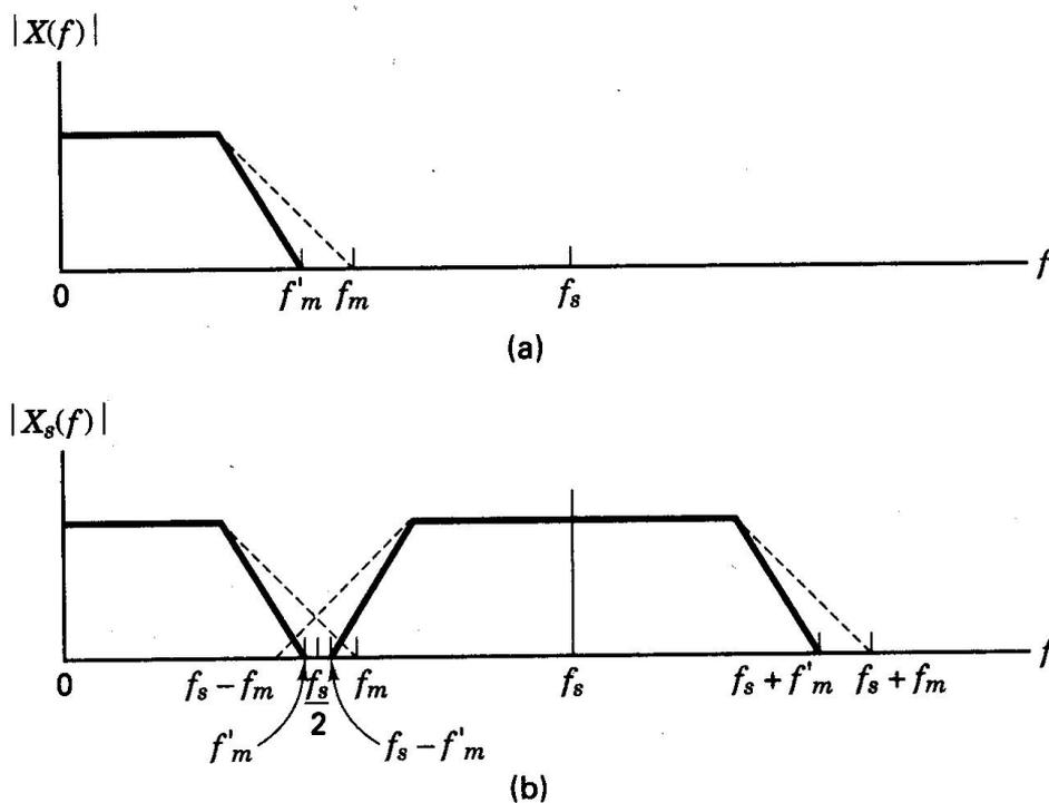
Figure 2.9 Prefiltering
