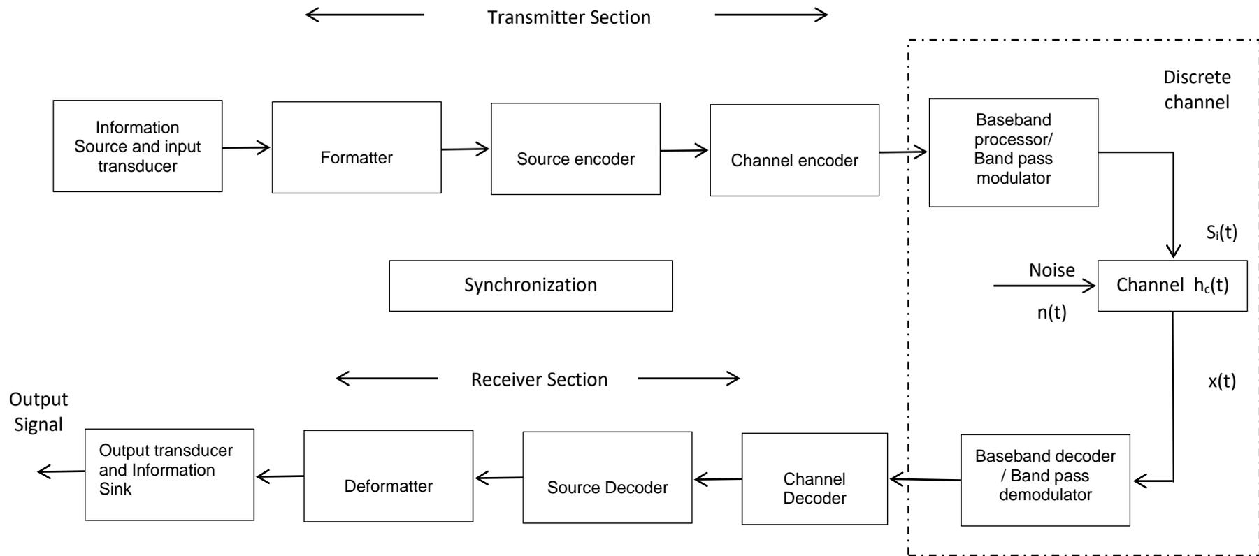
Figure 1.2(a): Block diagram of a Typical Digital Communication System
