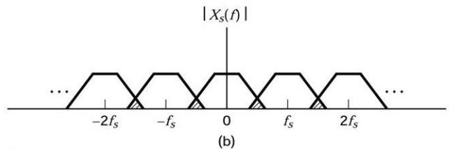
Figure 2.7 Sampled Spectrum for  $f_s < 2 f_m$
