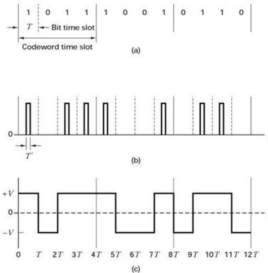
Figure 2.20 Example of waveform representation of binary digits
