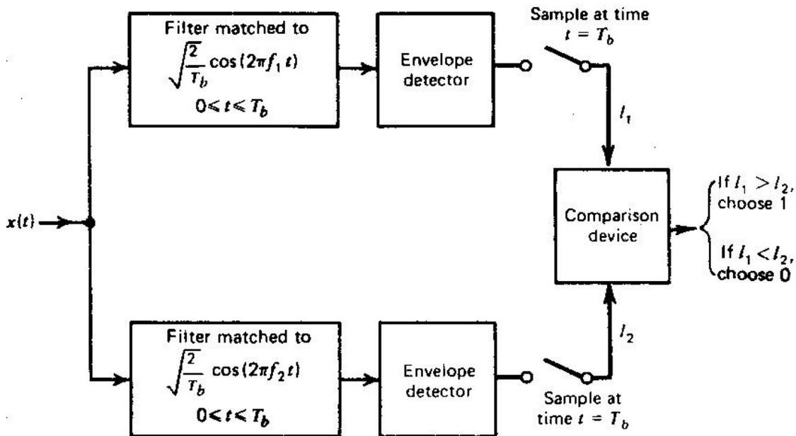
Figure 4.28 Non-coherent receiver for BFSK Digital communications
