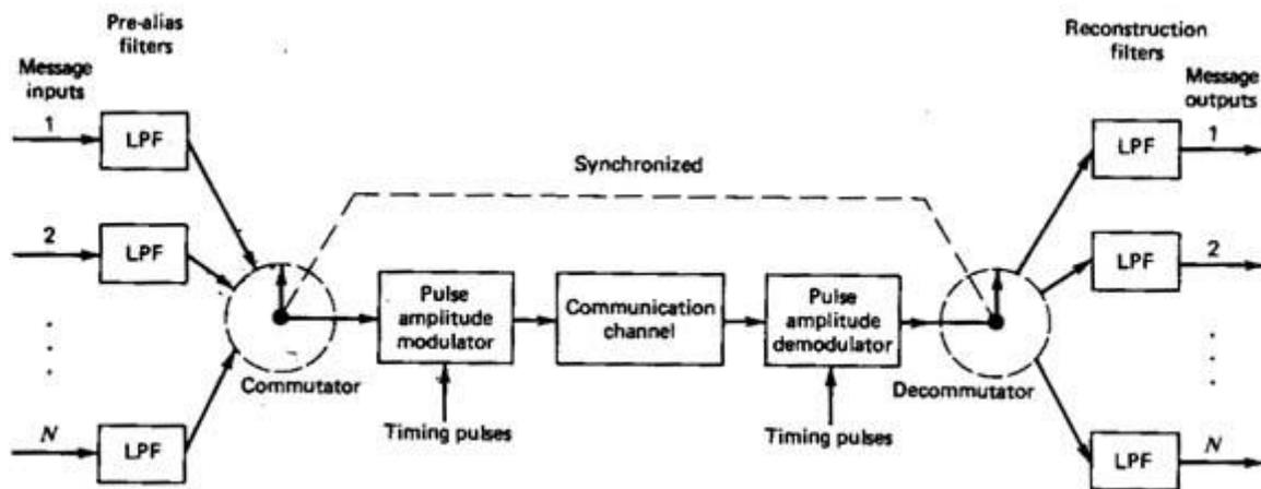
Figure 4.30 Block diagram of PAM / TDM system
