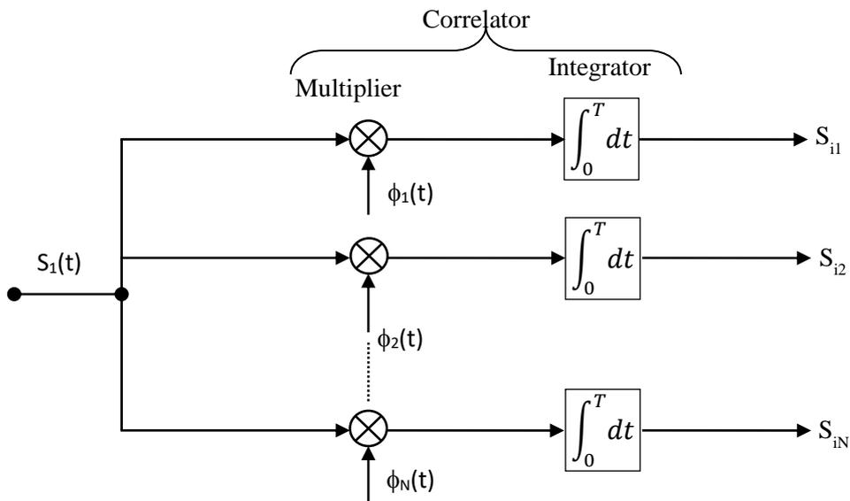
Figure 4.2 Scheme for generating the set of coefficients  $\{S_{ij}\}$
