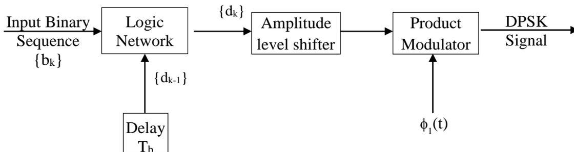
Figure 4.8 DPSK transmitter
