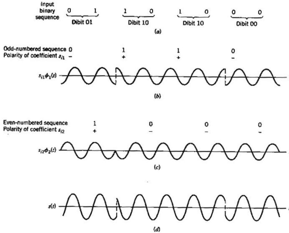
Figure 4.10 QPSK waveforms
