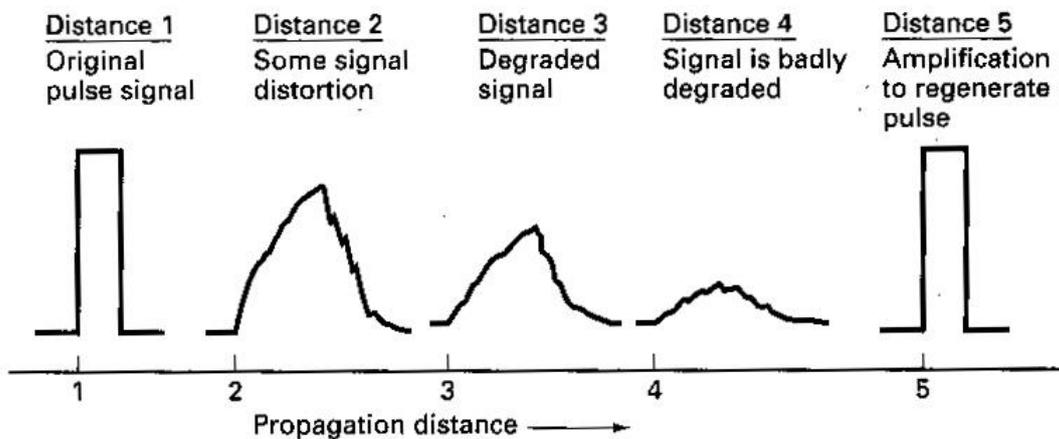
Figure 1.1 Pulse degradation and regeneration
