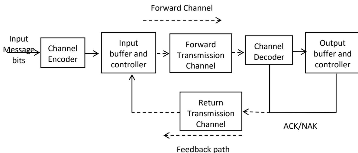
Figure 3.5 : Block diagram of basic ARQ system
