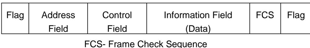
**Figure 1.14 Bit oriented Synchronous protocol**
