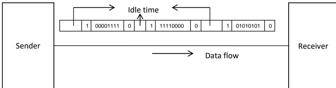
Figure 1.11 Asynchronous transmission
