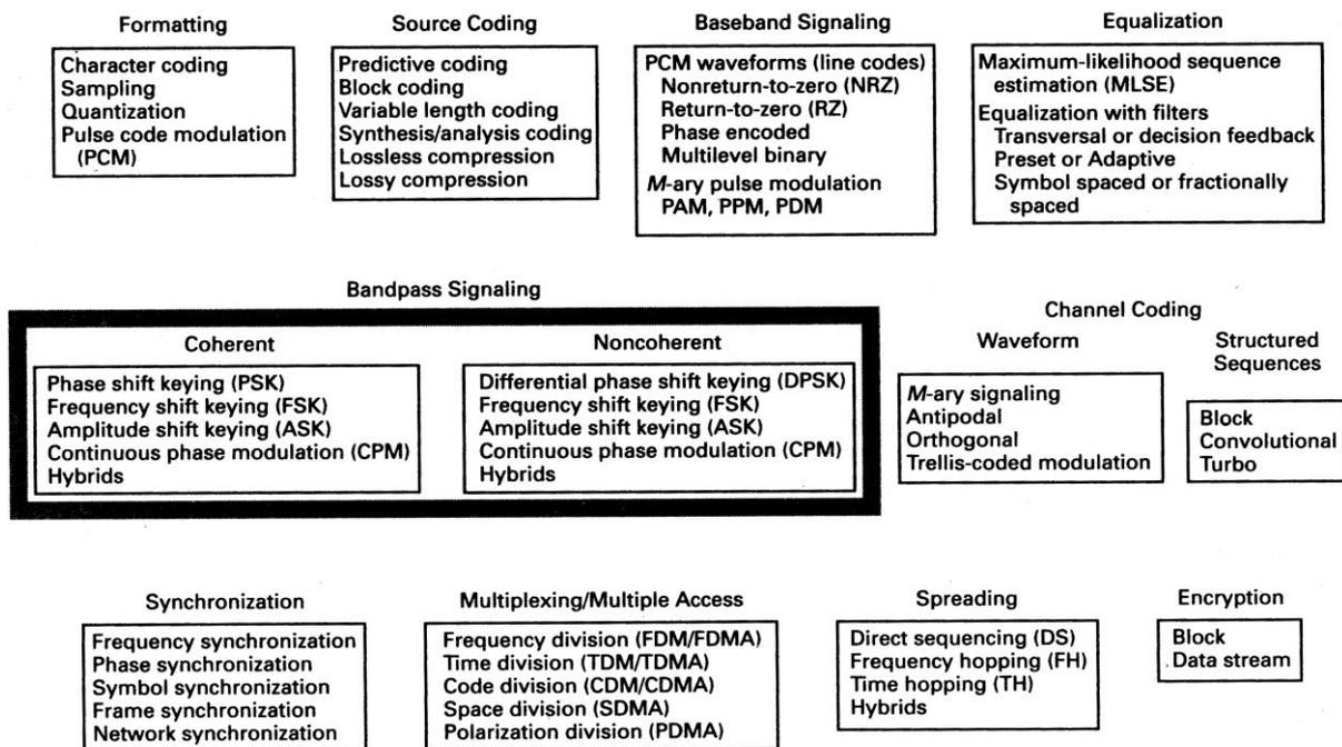
Fig. 1.2(b) Basic digital communication transformations
