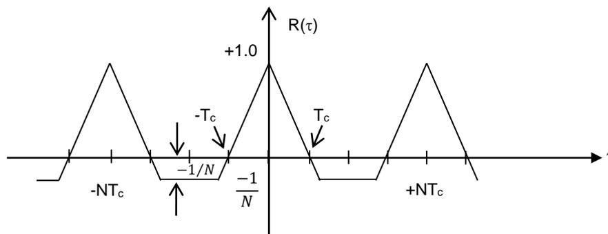
Figure 5.4 Autocorrelation function of a PN sequence
