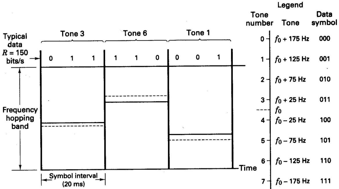
Figure 5.14 Frequency Hopping Example
