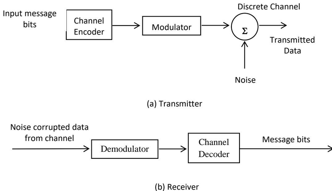
**Figure 3.1 Digital Communication System with Channel Coding**
