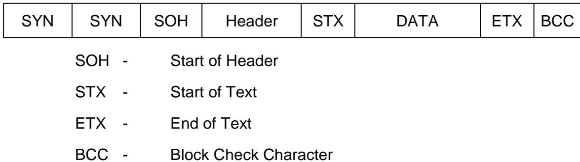
**Figure 1.13 Character oriented Synchronous Protocol**
