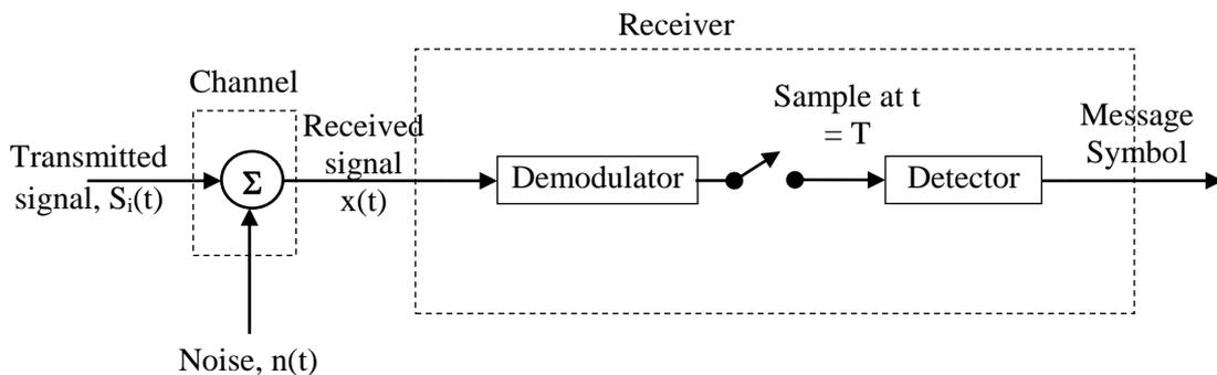
**Figure 4.19 Two basic steps in digital receiver**
