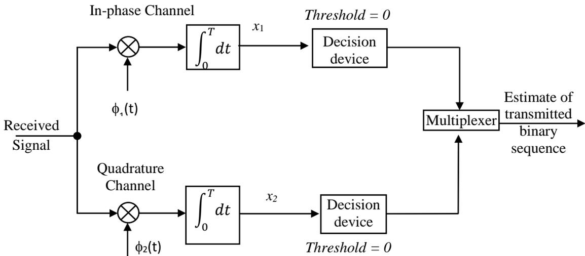
Figure 4.11 Coherent QPSK receiver
