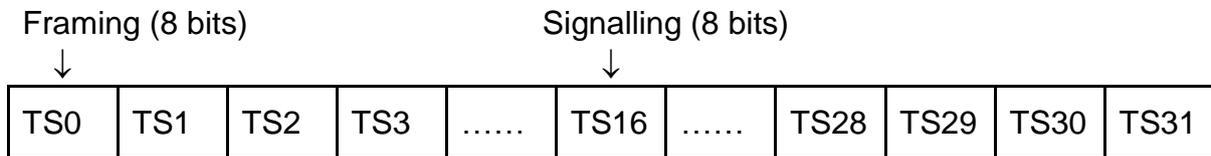
TS → Time slot each of 8 bits, one voice channel sample
