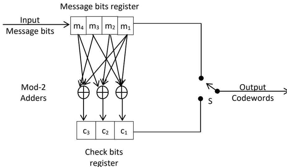
Figure 3.7 Encoder of (7, 4) Hamming code
