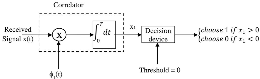
Figure 4.23 coherent binary PSK receiver
