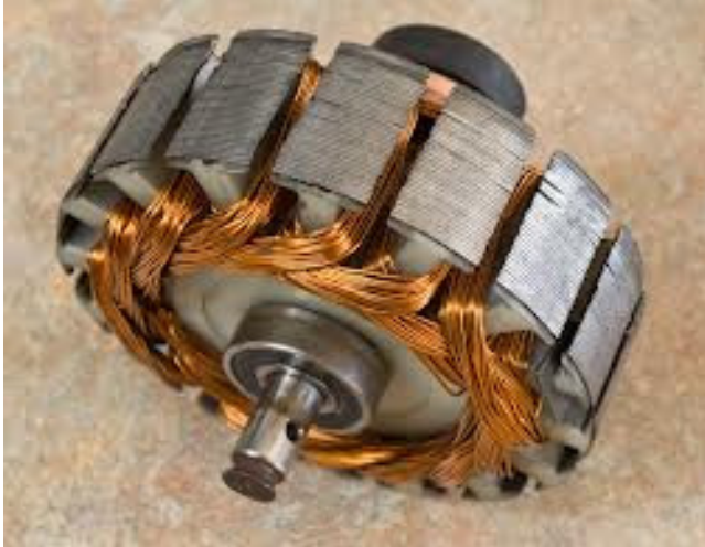
Armature core (rotor)
